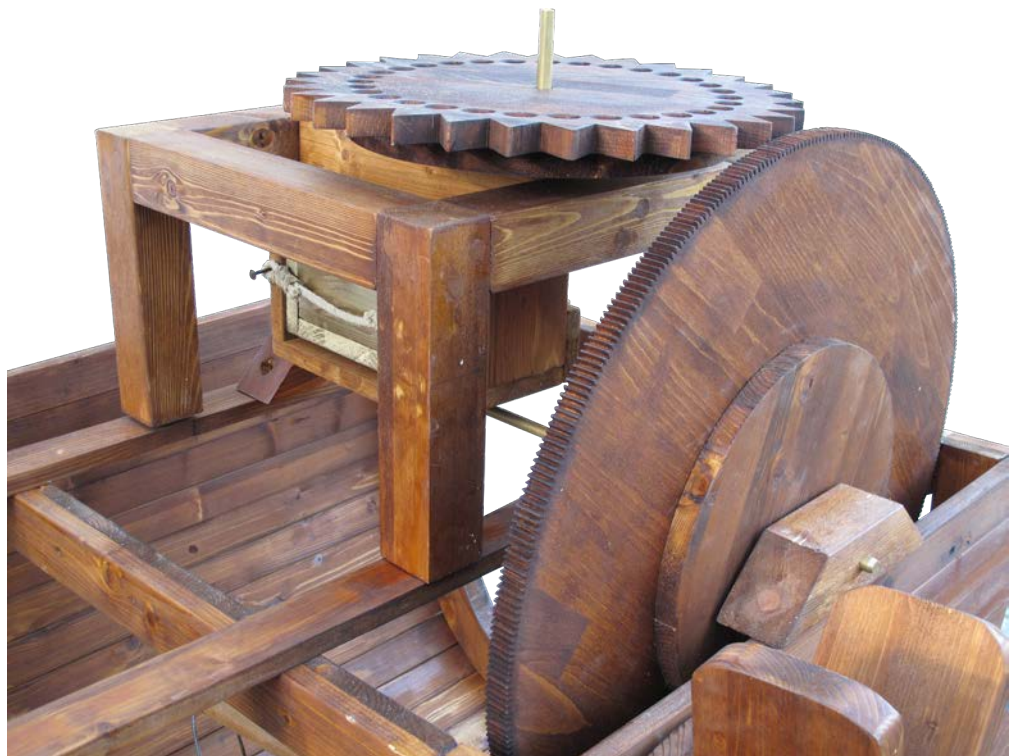
Part of a naval odometer – used to measure the distance travelled by sea.
